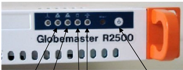
LAN2 LED LAN1 LED Disk LED Power LED ON/OFF Button
